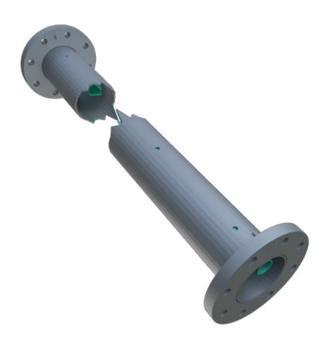
STAG «Dense Flow»: The technically and economically advantageous solution for dense-phase conveying of powdery bulk materials through pipes. A secondary air supply line with openings is located in the upper section of the conveying line. This design prevents or automatically eliminates blockages.
