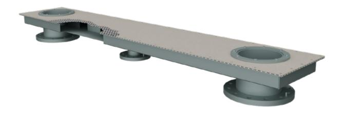
Fluid Channels are used in silos or bunkers where poorly flowing bulk materials are stored. The Fluid Channel is installed with a slight incline and, thanks to the large-area ventilation, even poorly flowing products are discharged without any problems.
