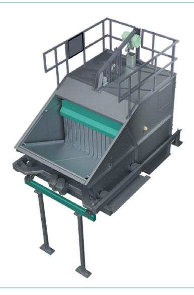
The use of a Coarse Particle Separator is suitable in a mechanical conveying process for bulk materials in order to separate out large particles (impurities). The advantages lie in the higher operational safety of the conveying system and its smaller dimensions downstream of the coarse particle separator.
