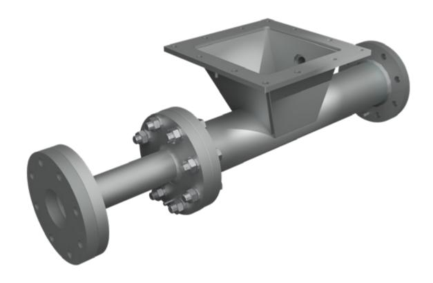
The injector is suitable for the pneumatic transport of non- or slightly abrasive products in thin-flow conveying systems. In combination with a rotary valve as a pre-seal, the dual function of dosing and pressure sealing is possible in a continuous product feed into the conveying line, resulting in a high level of operational reliability with minimal control effort. The different geometries of the range enable problem-free conveying of a wide variety of bulk materials.
