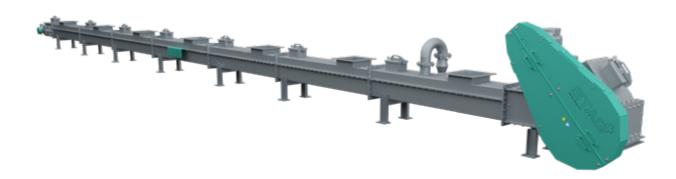
Trough Chain Conveyors are continuous conveyors and are suitable for transporting all types of bulk materials, including small-sized products and solid sludge. The advantages lie in the high temperature resistance, the low conveying speeds, especially with abrasive bulk materials and the robust and dusttight design. The possible applications and design variants are very versatile. More than 500 units are currently in use at over 100 satisfied customers.
