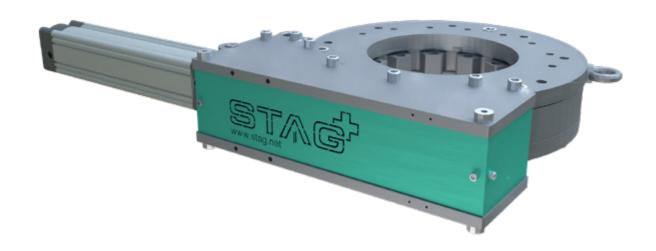
The «Silex» mechanical discharge aid is used for bulk materials that are difficult or impossible to fluidize. It is installed in silos, bunkers and containers of round or square design. Due to its low height and simple mode of operation, retrofitting in existing silos and containers is usually possible without major conversion work.
