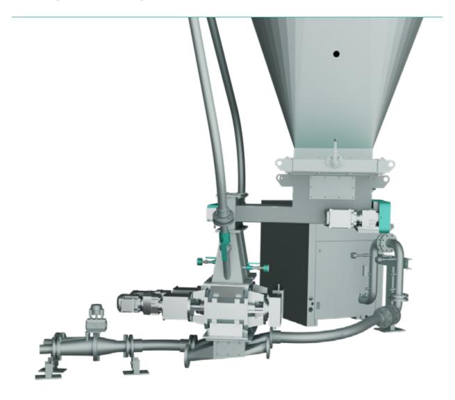
The system includes dosing, pneumatic conveying with the product-specific Air Blast Nozzle and the necessary air preparation. With volumetric dosing, the material is discharged exclusively by volume and therefore by quantity. This takes place via a multiple screw feeder, which is adjusted to customer specifications.
