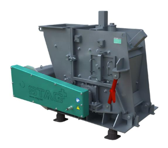
The Impact Mill has been specially developed for the comminution of agglomerations in bulk material. This application is primarily used for processing boiler ash from incineration plants. The adjustable impact mechanism crushes the bulk material to a particle size distribution that is not critical for pneumatic conveying. This is the prerequisite for ensuring a high level of functional reliability for pneumatic conveying, even with critical bulk materials.
